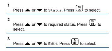
After a blinking cursor appears, press ↓ to move one space to the left or press ▶ to move one space to the right. Press ★ to delete any unwanted characters. Long press ♥ ⓑ to change the text entry method. Press ♥ ⓑ once editing is complete. The display shows Status Saved and radio returns to Status List.
