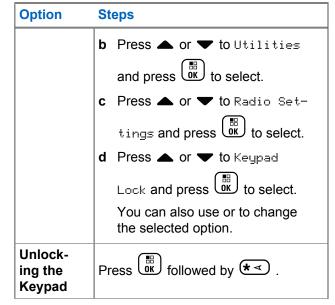
After the keypad is locked, the display shows Keypad Locked and returns to the Home screen.
